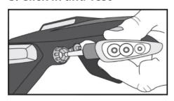
Click your new indicators into position and insert the rubber dust plug into the hole provided on the back of the indicator. This stops the plug flapping in the wind and further secures the indicator to the socket. Test your indicators.
