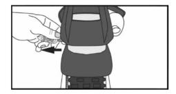
For off-road use, remove the dust plugs from the back of the light, unclick your indicators and stow. Ensure you reinsert the attached rubber dust plug into the socket whenever the indicators have been removed to avoid moisture, mud or dust entering the socket.
