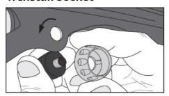
To ensure the socket is correctly installed on your bike, add/remove the included plastic spacers so the notch on the nut ends up flush with the top of the thread of the socket. If required, reduce the thickness of your bike's plastics with hi-grit sandpaper or dremmel tool (work from the inside of the plastic).
