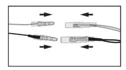
Join wires, Positive (red) to Active wire, then connect the Earth wire (black). Check with your motorbike manufacturer for wire diagram or a qualified motorcycle repairer.
