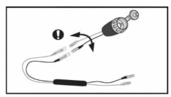
If you are converting from incandescent globe indicators to CLICKnRIDE® LED indicators, wire-in CLICKnRIDE® resistors as shown (sold separately). Install 1 resistor for each LED indicator until there is enough 'load' in the system to trigger the Flasher Unit. It is normal for the resistors to become hot to touch. Avoid placing them in contact with parts that may be effected by excess heat. Alternatively, replace your bike's Flasher Unit with an LED unit.
